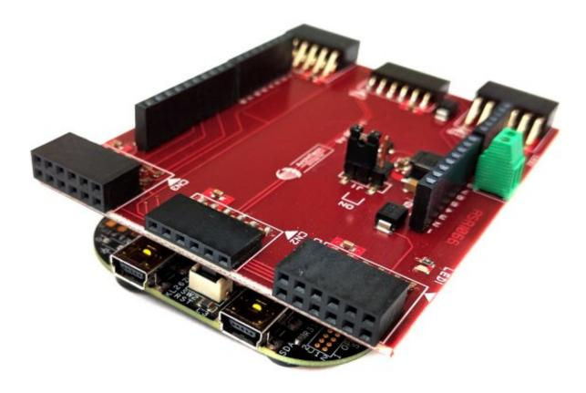
Connect the PMOD module to the CN7 then power supply the FRDM board via mini USB connection.
